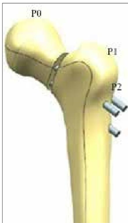
**Figure 2.** Loading points on femur**Table 2.** Compression values at the fracture side and maximum stress values on fracture side and implant
